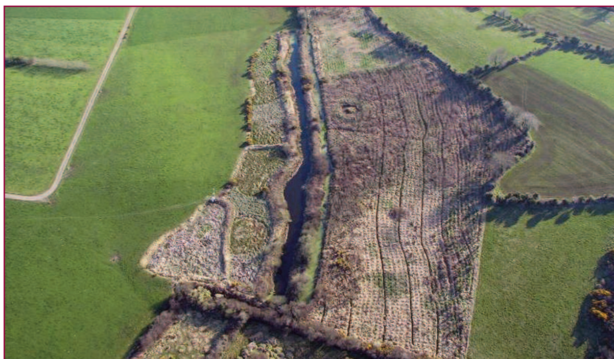
Fig 5.3 ICW showing landscape-fit; in this example the ICW configuration reflects the meandering of the adjacent water body
