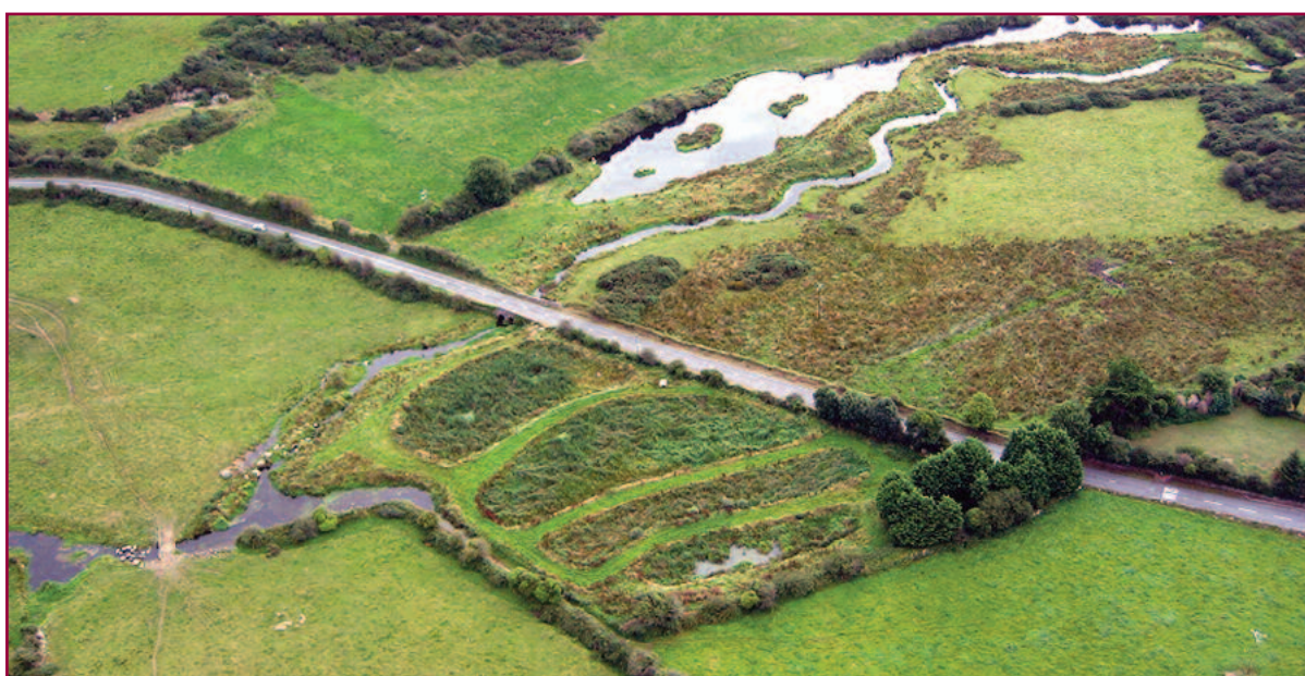
Fig 5.1 Aerial View of ICW showing curvilinear fit of segments/ponds to landscape contours
